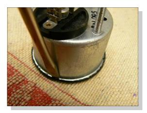
Careful separation allows the cover and glass to be removed and gives us exposure to the gauge itself. A handsome looking gauge if I do say so myself. Thank God we get to look at these all day instead of digital readouts of 14.14V! There's beauty in an old analog gauge as much as one can appreciate the craftsmanship of a Swiss Omega watch over it's cheap Korean digital counterpart. Long live Analog gauges!
