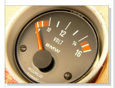
Now with a small fine tipped paint brush, we can carefully apply the paint just to the needle. Here's how it looks when finished.
