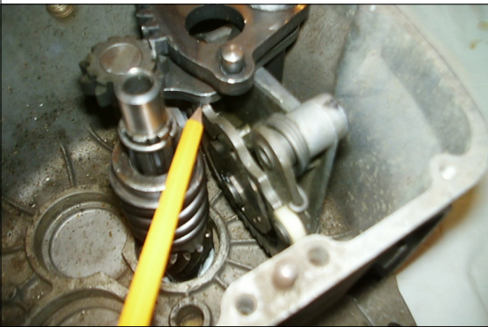
The gear selector is moved by a bent kickstart shaft
